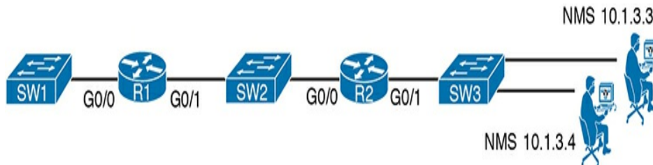
Figure D-12 Sample Network for SNMP Examples, with NMS at 10.1.3.3
