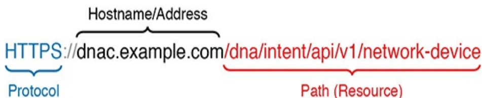
Figure 18-6 URI Structure for REST GET Request
